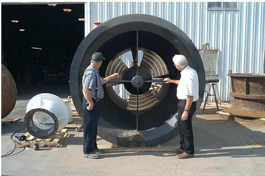
Fred Schantz, Sutter Mutual Water Company and Steve Greenwood, Durham Pump inspect new Pump #2 54" Johnson Pump Bowl and Impeller
